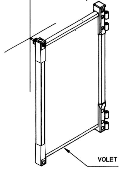
PERCER AVEC UN FORET DIA. 5 MM JUSTE LONG. 35 MM.
